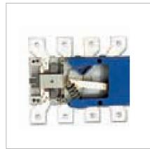
The moving contact mates with the fixed contact by a roll and slide movement of the moving contact assembly. The contact is first made with the arcing contact and thereafter with the main contact. During breaking, the arc formation is across the arcing contacts thereby protecting the main contacts which results into enhanced life of the switch. The arc is effectively quenched & confined by the set of arc chutes / arc barrier in each phase.
