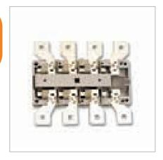
The switching mechanism is quick make, quick break type independent of the speed of the operation. There are four breaks per pole thereby resulting into faster quenching of arc. The load and line can be connected on either side by virtue of isolation on both the sides. The entire switching mechanism alongwith the fixed and moving contact assembly are housed in a polyester reinforced, moulded frame/cover, having high dielectric strength & thermal withstand capacity.
